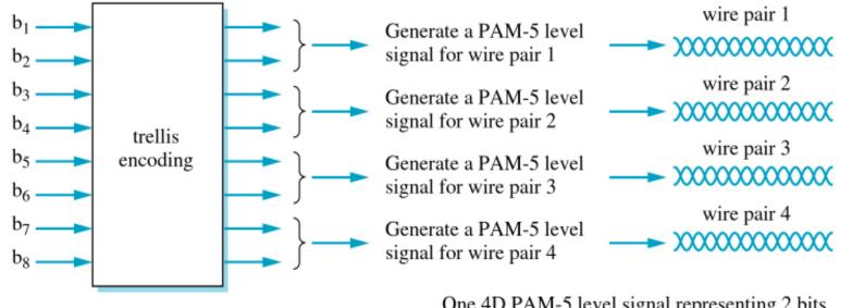
One 4D PAM-5 level signal representing 2 bits on each wire every 8 ns. 250 Mbps per wire pair.
