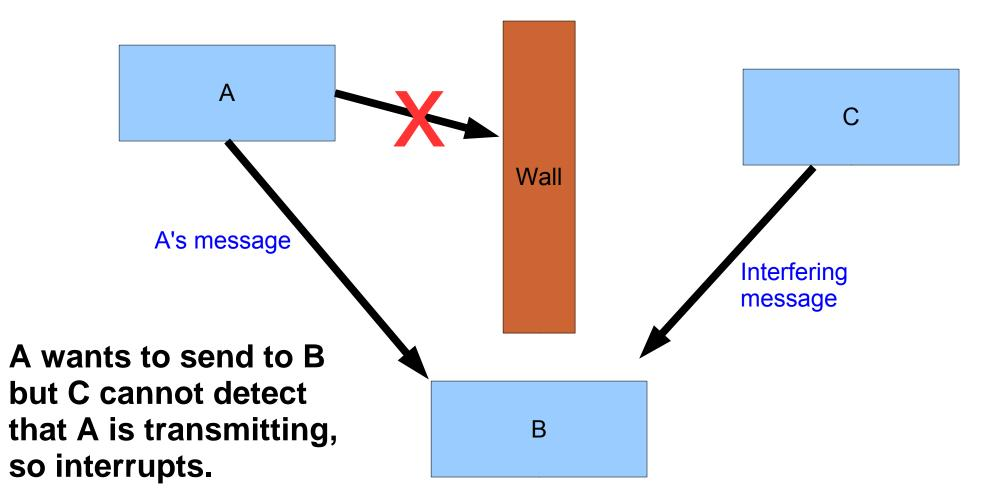
Solution: A and B exchange short "request to send" and "clear to send" packets. C missed the RTS but hears the CTS and keeps quiet. (Optional and not found on cheaper equipment.)
