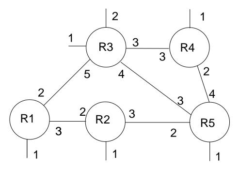
The routers are named R1 to R5 and each one has its interfaces numbered starting from 1. They have the following (fictional) IP addresses:
