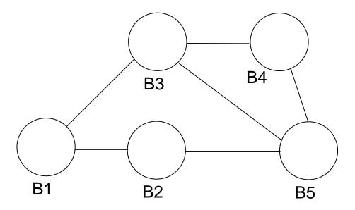
Assume B1 is elected as the root bridge. Assuming the link metrics are all the same, list the links in a valid spanning tree (e.g. B1-B2, etc.). Which link(s) will not be used? [4 marks]
