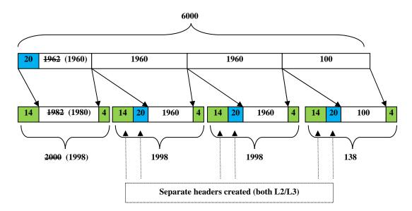
Overhead will increase: Instead of one packet, we are now sending four packets, each with 20 bytes + 18 bytes (of headers). In other words,  $3 \times 38 = 114$  bytes more data transmitted; lowering the link effective data transport rate.
