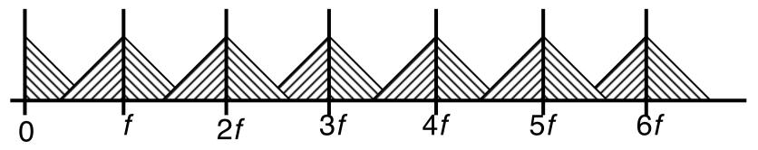
• Clearly, if the sampling frequency  $f \ge 2w$  (*w* is the signal bandwidth) there is no interference; the sampling is unambiguous and the original signal can be reconstructed.
