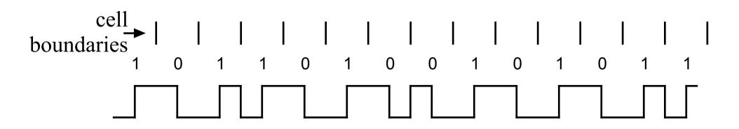
**Differential Manchester Encoding** The centre of each bit cell has a transition; a 0 bit starts with a transition at the cell boundary, while a 1 bit has no leading transition.
