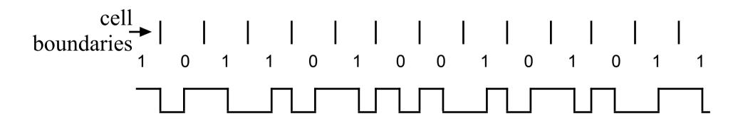
**Frequency Modulation (FM)** A transition at every cell boundary and at the middle of every "1" cell. Also known as Binary FM, Phase-Encoding Mark or Double-Frequency
