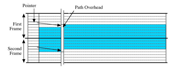
• The AU Pointer of the section header gives the byte offset within the physical frame of the start of the data frame (the first byte of the Path Overhead)
