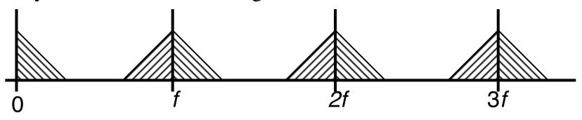
• With a very low sampling frequency the teeth are more closely-spaced and the sidebands interfere. The samples are ambiguous, with a mixture of components from the correct signal and the adjacent sidebands. The data cannot be recovered.
