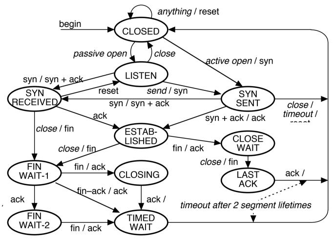
Labels on the transitions show the "input or actions / output" (output may be empty).
