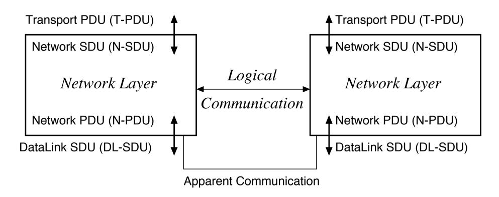
• Note that the *same* message is a *Protocol Data Unit* (PDU) above the layer boundary and a *Service Data Unit* (SDU) below the boundary.
