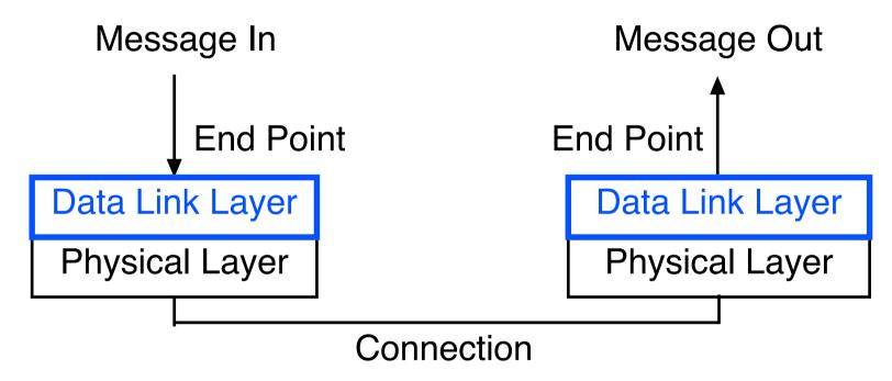
• Problems of assembling bits into bytes, indicating start and finish of message, handling lost or corrupted data
