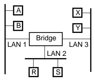
The network starts from a completely idle state, with no entries in the bridge's routing tables.
