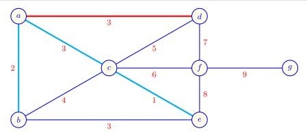
**Step 4:**  $\{S_a = A.\mathtt{set}(a)\} \neq \{S_d = A.\mathtt{set}(d)\}; \text{ add } (a,d); A.\mathtt{union}(S_a,S_d)$ Disjoint-sets ADT  $A = \{\{a,b,c,d,e\}, \{f\}, \{g\}\}\}$
