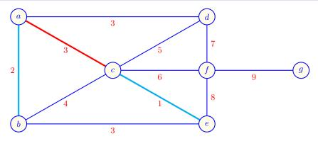
**Step 3:**  $\{S_a = A.set(a)\} \neq \{S_c = A.set(c)\}; add(a,c); A.union(S_a, S_c)$ Disjoint-sets ADT  $A = \{\{a, b, c, e\}, \{d\}, \{f\}, \{g\}\}\}$
