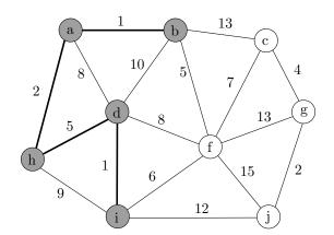
$$S = \{ \frac{a, b, d, h, i}{a} \} \qquad w = \begin{bmatrix} \frac{a}{a} & b & c & d & f & g & h & i & j \\ \hline 0 & 1_a & 13_b & 5_h & 5_b & \infty & 2_a & 1_d & 12_i \end{bmatrix}$$
