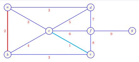
**Step 2:**  $\{S_a = A.set(a)\} \neq \{S_b = A.set(b)\}; add (a, b); A.union(S_a, S_b)$ Disjoint-sets ADT  $A = \{\{a, b\}, \{c, e\}, \{d\}, \{f\}, \{g\}\}$
