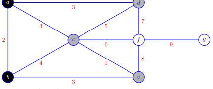
$$\text{adjacent } x \in \{d, e, f\}; \ \underline{x} \leftarrow \underline{e}; \ \underline{\text{key}_e = 3 > \text{cost}(c, e) = 1}; \ \text{key}_e \leftarrow 1$$
