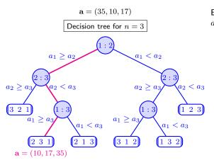
Example:  $a_1 = 35, a_2 = 10, a_3 = 17$ Comparison 1:20  $(35 > 10) \rightarrow$ left branch  $a_1 > a_2$ Comparison 2:32  $(10 < 17) \rightarrow$ right branch a2 < a3 $\bigcirc$  Comparison 1 : 3:  $(35 > 17) \rightarrow$ left branch a1 > a34 Sorted array  $231 \rightarrow$  $a_2 = 10, a_3 = 17, a_1 = 35$  **Lemma:** A decision tree of height h has at most  $2^h$  leaves.
