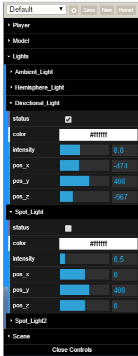
Fig-32: GUI light controls - directional light and spotlight
