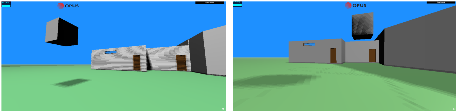
Fig-41: Inconsistencies in rendering shadows within within scene - random shadows on model (left; random shadows on ground and cube (right)
