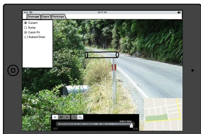
Fig 3. Inventory Validation—Misplaced Culvert
