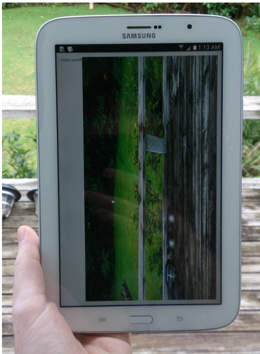
Fig 26. Camera working incorrectly when rotated
