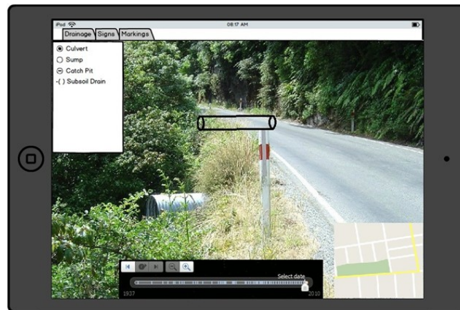
Fig 7. Inventory Validation—Misplaced Culvert
