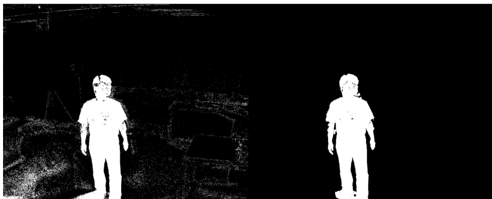
Figure 3.2: left: silhouettes with noise and shadow. right: silhouettes after shadow and noise removal
