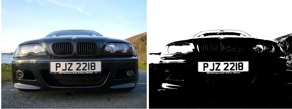
Figure 1.4: Example of Otsu binarization. Left: Original image [24]. Right: Result of Otsu's binarization.
