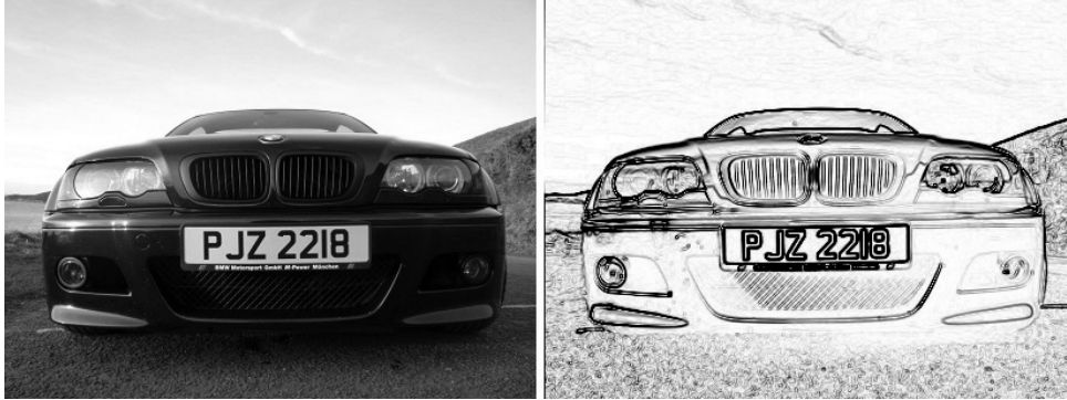
Figure 2.2: Left : Grey-level input image. Right : Result after applying the Sobel operator.
