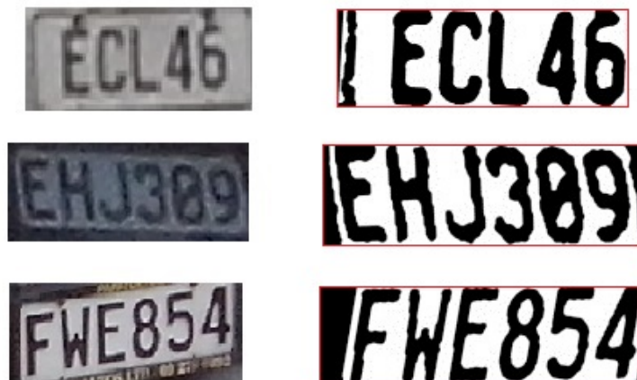
Figure 3.14: Left : Tilted view plates. Right : Tilt corrected, ready for extraction.
