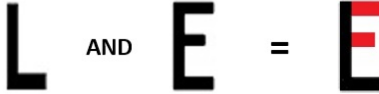
Figure 4.4: Example of problem faced using AND operator. Letter 'L' detected as an 'E'.
