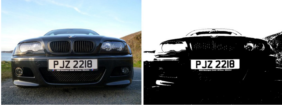
Figure 2.4: Example of Otsu binarization. Left: Original image [25]. Right: Result of Otsu's binarization.
