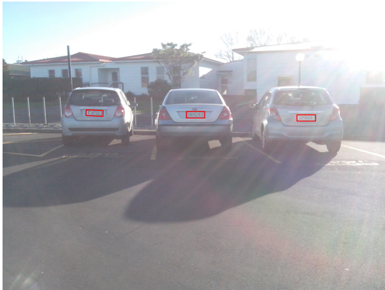
Figure 3.4: Successful detections with high exposure to sunlight.
