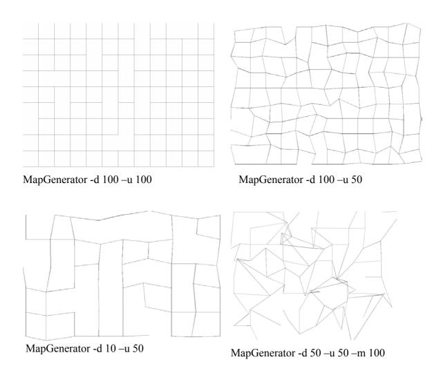
Currently outputs with high movement, like the bottom right example, are not recommended. This is due to the fact that an error in the checking of overlapping roads means that some will not have a node placed at their overlapping point. This creates a city that is 'layered' in parts – such cities are not considered reasonable.
