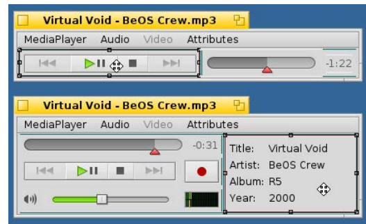
Figure 3. Examples for layout customization of the Media Player. Top: the interface was reduced to only a few widgets. Bottom: a record button and an MP3 tag view were added and the layout was rearranged.
