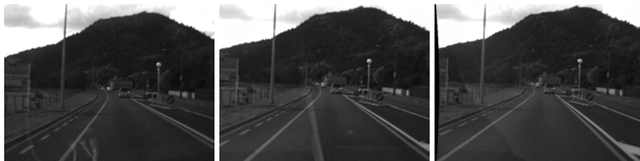
Fig. 1. Three frames of image sequences taken with cameras (called: third , left , and right camera - from left to right) installed in HAKA1, test vehicle of the .enpeda. project. Note the reflections on the windscreen, and differences in lightness (e.g., image of right camera is brighter than the other two). Left and right views are rectified.
