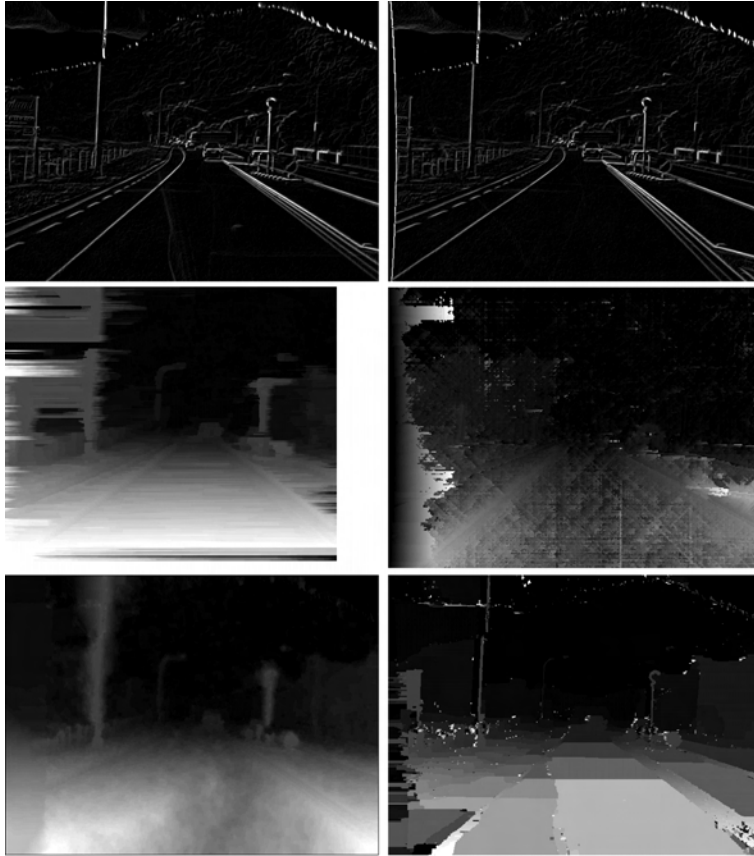
Fig. 4. Top: Sobel edge maps of the left-right stereo pair in Figure 1, used as stereo input pair. Middle: depth maps of single line DP (left) and Birchfield-Tomasi cost function in 16-ray DP (also known as SGM BT). Bottom: BP (left) and GC results.
