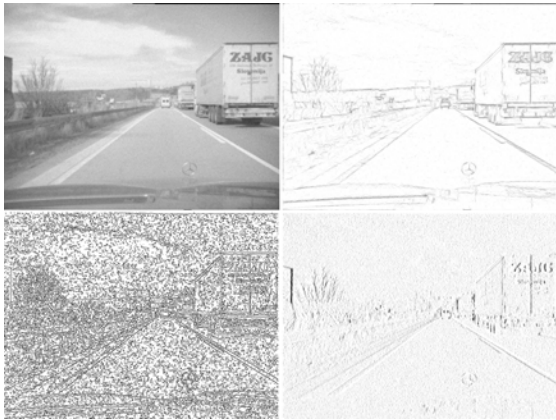
Figure 6: Construction-Site sequence image, number 179. Top row: noise added image and Kovesi-Owens edge image. Bottom row: Canny and Sobel edge images.
