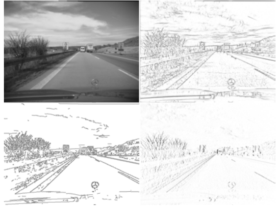
Figure 1: Construction-Site sequence [1], image number 31. Top row: original and Kovesei-Owens edge image. Bottom row: Canny and Sobel edge images.
