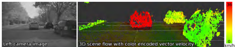
Fig. 1. Scene flow example. Despite similar distance from the viewer, the moving car (red) can be clearly distinguished from the parked vehicles (green).
