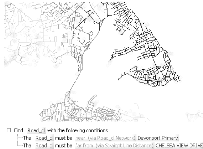
Fig. 3. Screenshot of the transparency method (top) used to visualise results of a qualitative query (bottom). The qualitative terms used to specify criteria (“very near”, etc.) capture the concept of vagueness and are accessible to non-experts in GIS.
