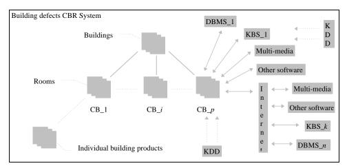
The many different types of fault would require substantially different case structures, and these might be arranged in a general-to-specific hierarchy. Each element of the hierarchy could consist of a 'cluster' or mini-case-base specific to the problem area ( $CB_i$ ). Each cluster might be augmented with a KBS, for instance the extant BREDAMP which diagnoses causes of dampness. In this manner, each 'element' of an object hierarchy would be populated by its own case base of context-
