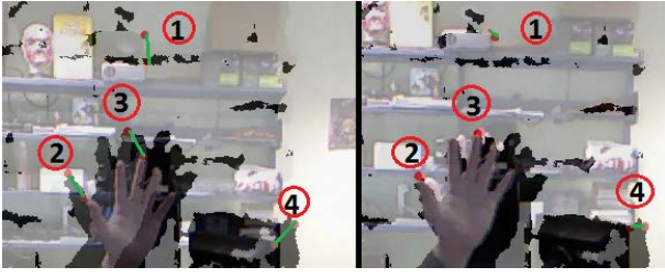
Figure 3: The depth image (grey scale) is overlaid with: (left) the original colour image and (right) the corrected colour image.
