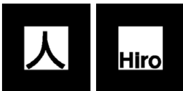
Figure 3: Example fiducial markers used with ARToolkit.
