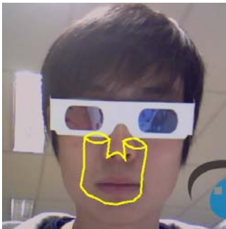
Figure 2: Inaccurate tracking with FaceAPI when anaglyph glasses are worn. The predicted face positions are indicated by the yellow outline.
