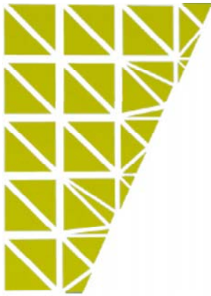
Figure 15: Triangulation around a diagonal cutting plane.
