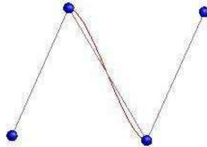
Figure 7: An example of a cubic Catmull-Rom Spline curve which is generated by four control points.
