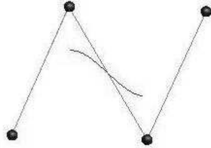
Figure 6: An example of a cubic B-Spline curve which is generated by four control points.
