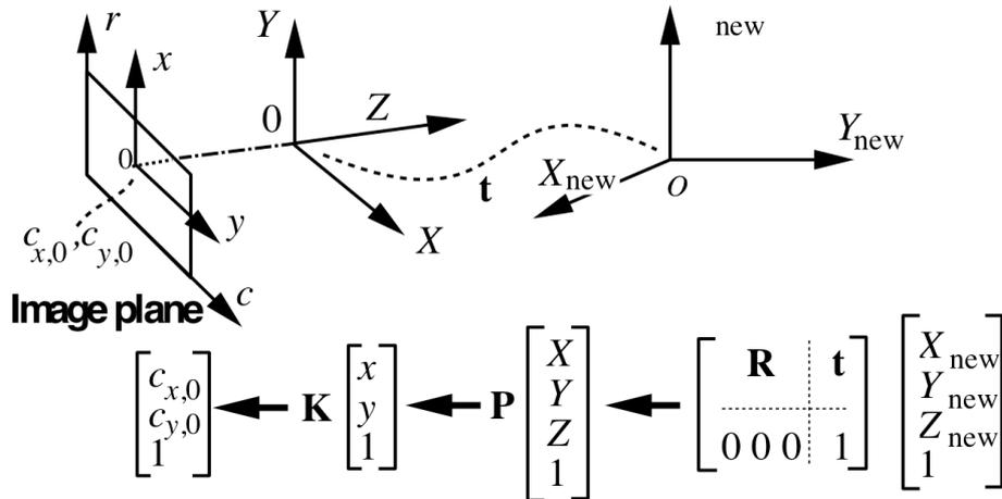
By combining co-ordinate transformations and projection in the camera coordinate system, one obtains a general perspective projection matrix for projecting a 3D point in the world coordinates onto the digital image:
