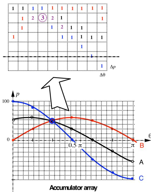
Figure 1.3: Implementation of the Hough transform.
