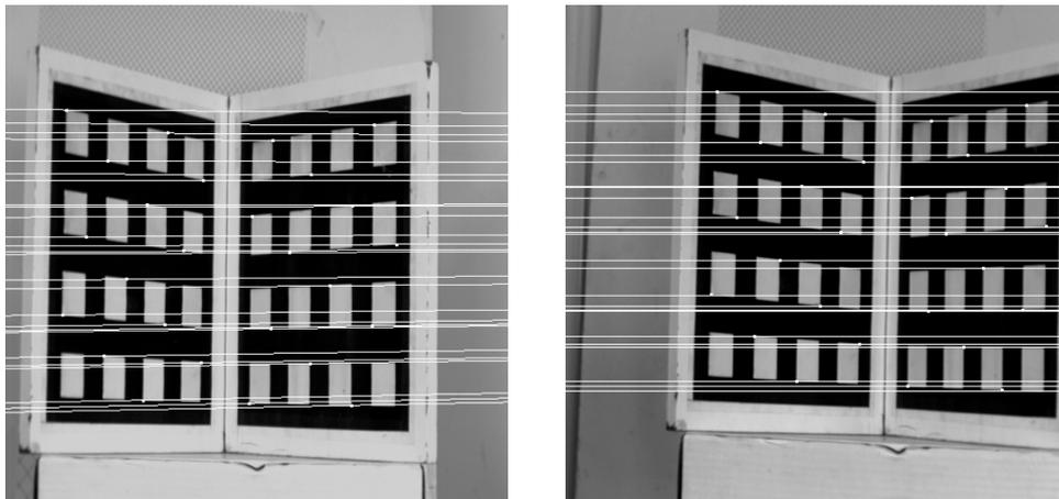
Figure B.3: Epipolar lines for the matrix of Eq. B.9 (the mean square distance error: 0.02 pixel, the maximum square distance error: 0.138 pixel).
