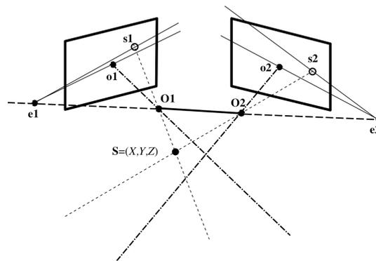
Figure 2.9: Binocular viewing and fundamental matrix.
