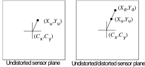
Standard calibration procedures account for only a first order radial lens distortion described by non-linear model with a single distorting parameter,  $\kappa_1$ . The coefficient  $\kappa_1$  relates the distorted (true) and undistorted (ideal) image coordinates as follows:
