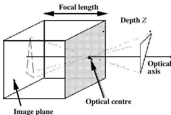
Figure 2.2: Pin-hole camera.
