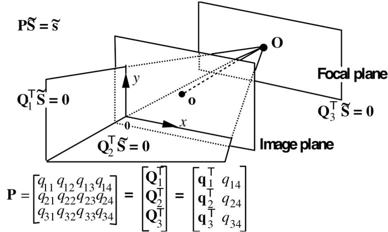
The standard CRF has the  $X$ - and  $Y$ -axes parallel to the  $x$ - and  $y$ -axes of the image, respectively. The  $Z$ -axis coincides with the optical axis of the camera that is perpendicular to the image plane and goes through the optical centre.
