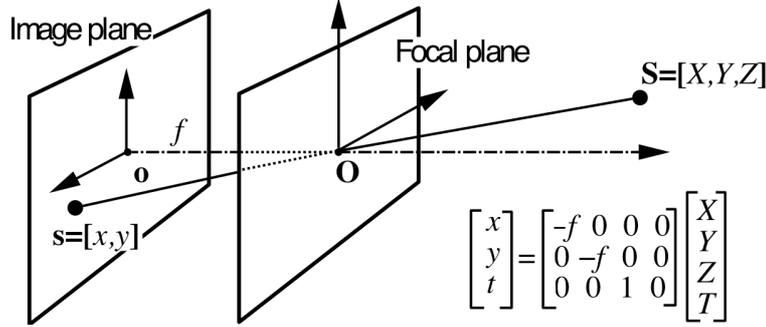
Perspective projection is a relationship between the image and 3D spatial coordinates in the standard CRF (coordinate system of the camera):
