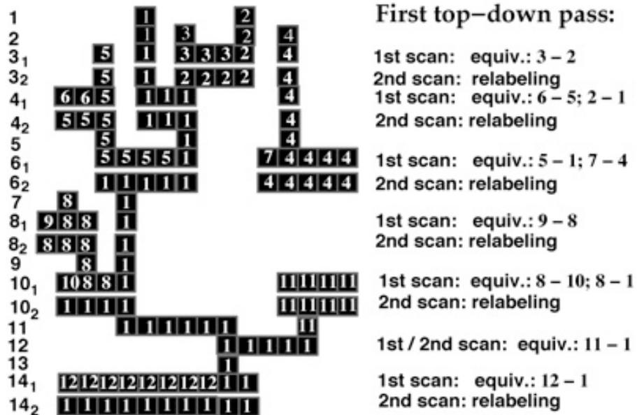
Figure 4.4: Space-efficient labeling: first top-down pass.
