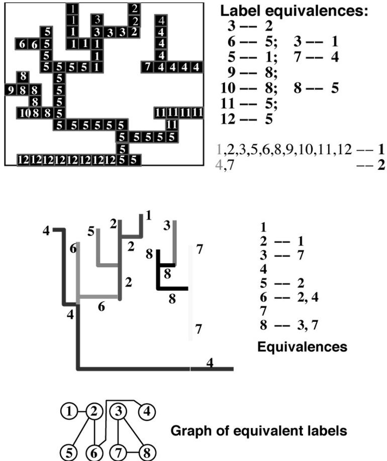
Figure 4.2: One more example of the connected components labelling.
