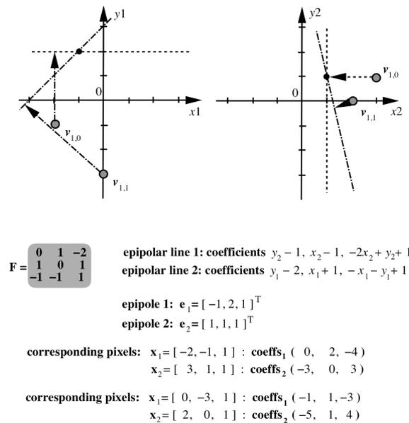
Figure 2.13: Changes of the epipolar lines in Fig. 2.11 for the new epipoles' ( $e$ ) position..
