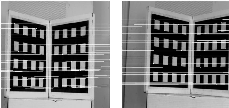
Figure B.2: Epipolar lines for the matrix represented by Eq. B.8 (the mean square distance error: 0.02 pixel, the maximum square distance error: 0.145 pixel).
