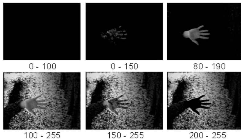
Figure 3.4: Segmentation with a range of thresholds.
