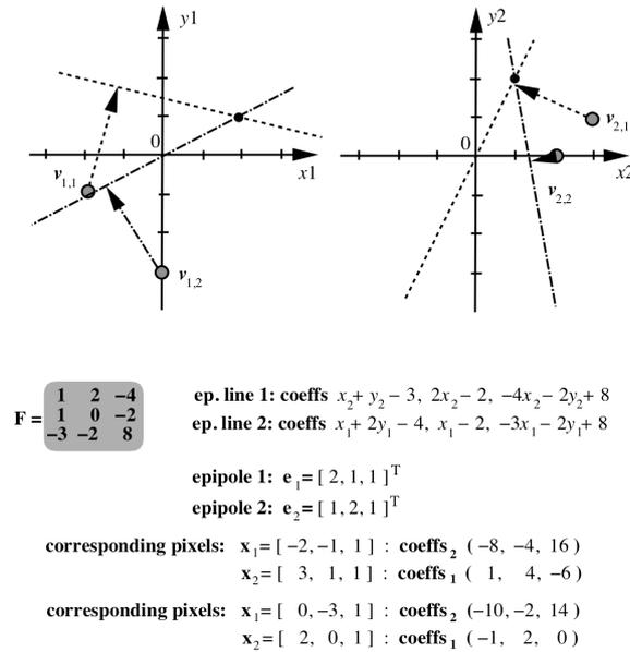
Figure 2.12: Changes of the epipolar lines in Fig. 2.11 for the new parameters  $a$ .
