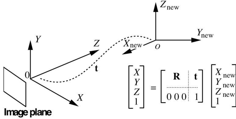
The matrix  $\mathbf{R}$  and the vector  $\mathbf{t}$  describing the orientation and positioning of the camera with respect to the new WCF (world co-ordinate frame) are called **extrinsic** camera parameters.
