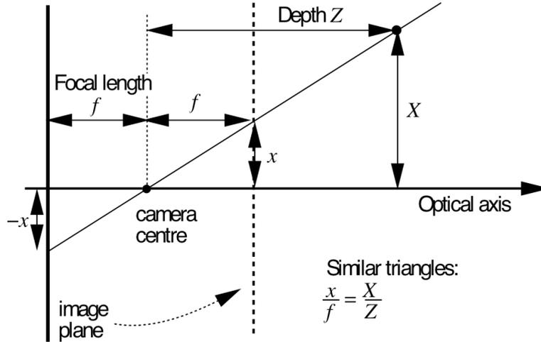
Figure 2.4: Pin-hole camera model.
