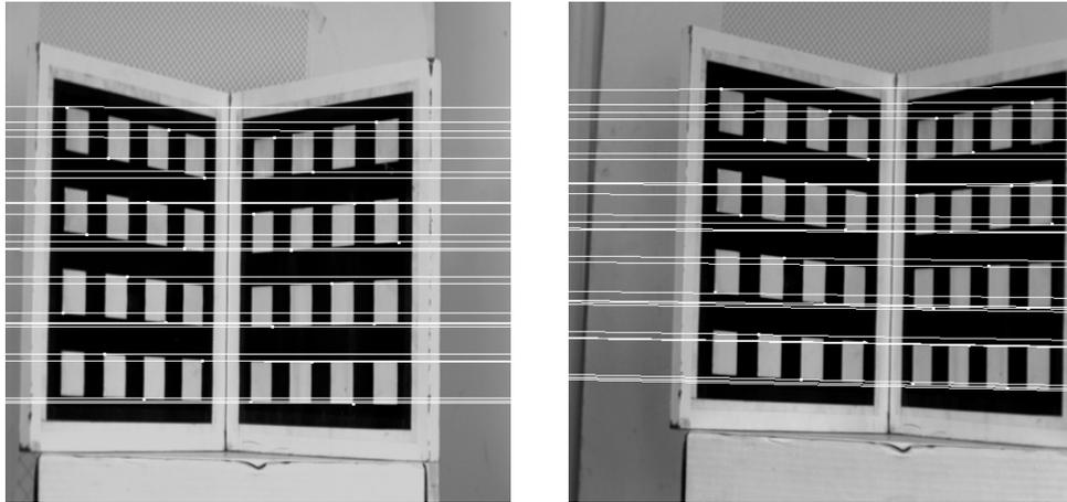
Figure B.1: Epipolar lines for the matrix represented by Eq. B.6 (the mean square distance error: 0.01 pixel; the maximum square distance error: 0.122 pixel).
