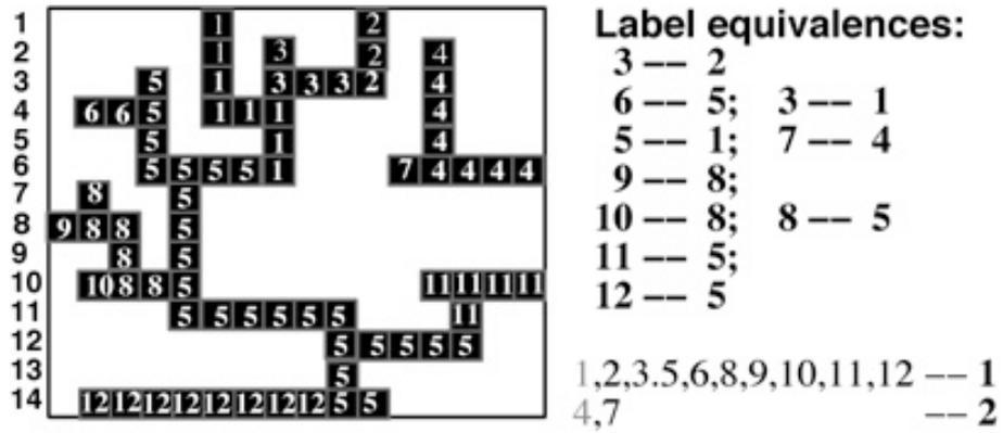
Figure 4.3: Space-efficient labeling: label equivalences.
