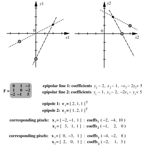
Figure 2.11: Corresponding pixels  $\mathbf{s}_{j,k}$ ,  $j = 1, 2$ ;  $k = 1, 2$ , and epipolar lines under given parameters  $\mathbf{a}$ ,  $\mathbf{e}$ .
