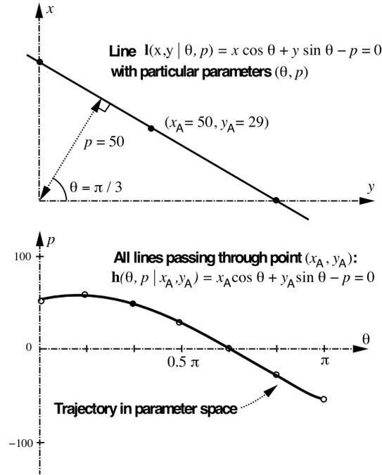
Figure 1.1: Hough transform.
