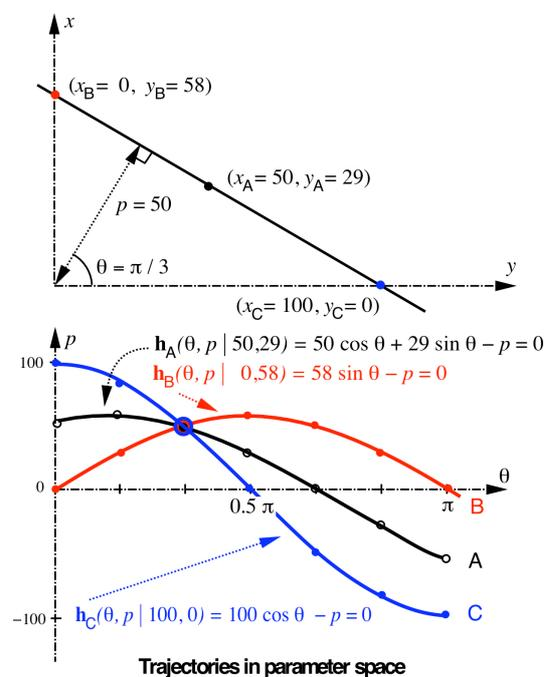
Figure 1.2: Hough transform: intersecting trajectories.
