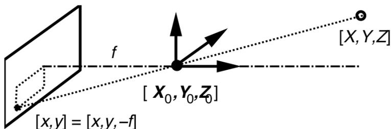
Figure 2.3: Pin-hole projection.
