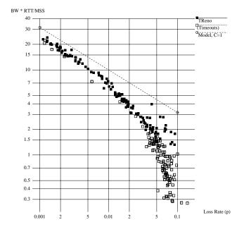
Figure 9: TReno measurement data This data fits Equation 3 with  $C=0.744\pm0.193$  or to Equation 5 with  $k=-0.617, C=0.375\pm0.054$ . These are poorer than the fits in Table 4, in part because the TReno data extends to much worse loss rates, where the effects of rounding become more pronounced. The C values are lower, indicating about 20% lower performance than TCP in a simulator.
