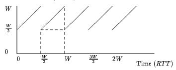
Figure 1: TCP window evolution under periodic loss Each cycle delivers  $(\frac{W}{2})^2 + \frac{1}{2}(\frac{W}{2})^2 = 1/p$  packets and takes W/2 round trip times.
