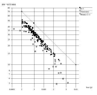
Figure 10: Measured TCP data, Set 1 This data fits Equation 3 with  $C=0.700\pm0.057$  or to Equation 5 with k=-0.525,  $C=0.574\pm0.045$ . These values for C are about 25% lower than TCP in a simulator.
