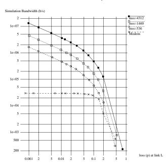
Figure 15: Effect of loss rate at link L.
