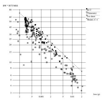
Figure 11: Measured TCP data, Set 2 This data fits Equation 3 with  $C=0.908\pm0.134$  or to Equation 5 with  $k=-0.611, C=0.418\pm0.058$ . Some of the individual data points are above the C=1 reference line. The live Internet measurements were not over long enough intervals to permit trimming the Slow-start overshoot described in Appendix B. This data set may have been subject to Slow-start overshoot.
