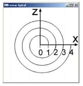
The parametric equation of the spiral is obtained by starting with the equation of a circle (with 3 revolutions) and then using a radius a function which increases linearly from 1 to 4. Hence we get:
