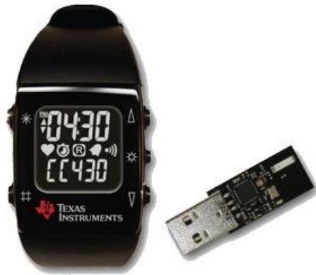
Figure 6. The eZ430-Chronos watch and USB dongle. This watch is what dWatch is based on. Reprinted from [3].
