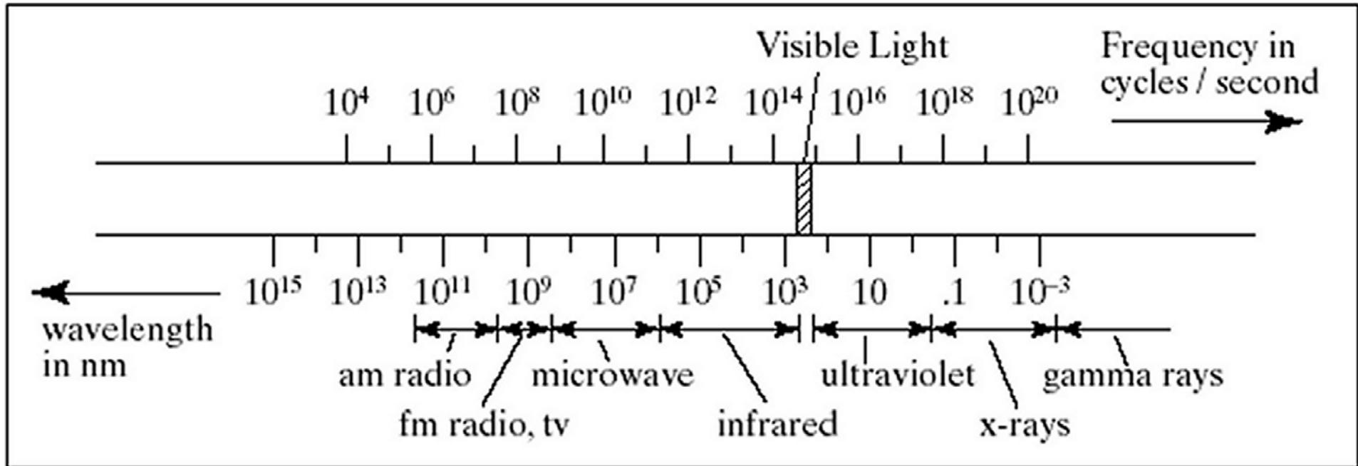
**FIGURE 12.1** Electromagnetic spectrum.
