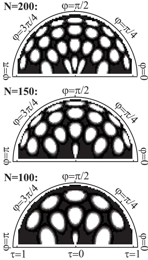
Figure 4: Likelihood in steps of grey (0=black, 1=white) as a function of  $\tau$  and  $\varphi$  when testing with the Mach-Zehnder interferometer of Fig.2. Each region demarcates the confidence area deduced from an experimental result. The number of distinguishable samples increases linearly with the number  $N$  of test particles per sample. Plots are for  $N = 100$ ,  $N = 150$  and  $N = 200$ .
