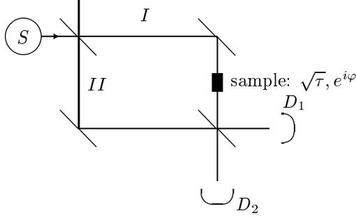
Figure 2: A particle emitted from source  $S$  impinges on the Mach-Zehnder interferometer where it can follow path I or path II. The particle can be detected in  $D_1$ , in  $D_2$ , or be absorbed in the sample.
