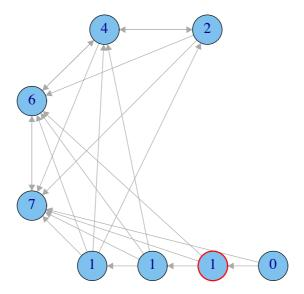
Figure 1: The principle behind the network topology used in the experiment. Labels on the nodes indicate the number of incoming links. The nodes have been divided in two groups. Each of the bottom nodes has only one feeding node, and those closer to the left feed increasingly more nodes above. The bottom nodes are not influenced by the nodes above.
