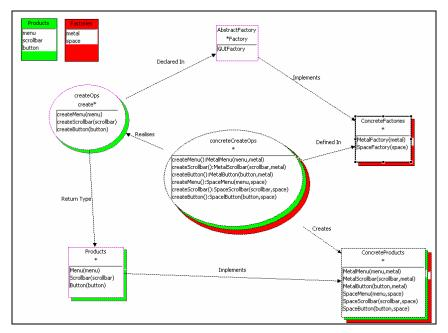
Figure 10: Instantiation Diagram for GUIFactory
