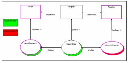
**Figure 6: Specification Diagram for the Adapter Pattern**
