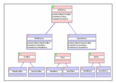
Figure 11: UML Design for GUIFactory
