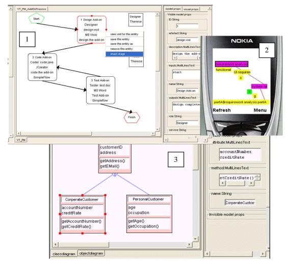
Figure 1. Some examples of DSVL tool diagrams.
