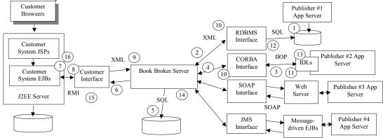
Figure 3. Architecture of our integrated system.
