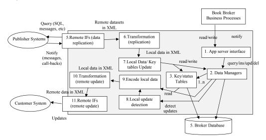
Figure 4. Broker architectural components.
