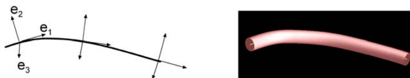
Fig. 1. The trajectory of a virtual nerve fiber tract is a cubic B-Spline curve (left). Using a low torsion reference frame we can fit a cylinder around it which defines the thickness of the fiber tract (right).
