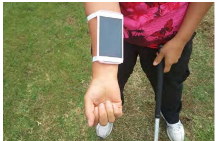
Fig. 3. Smartphone attached to the upper hand for measuring wrist acceleration.
