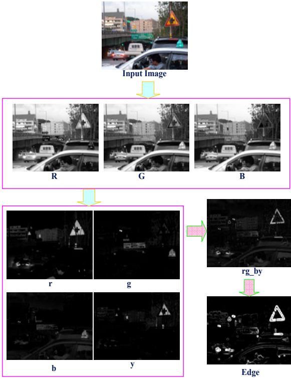
Fig. 2. The procedure of extracting edge and color features
