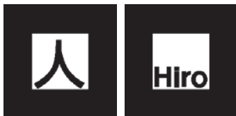
Figure 3: Example fiducial markers used with ARToolkit.
