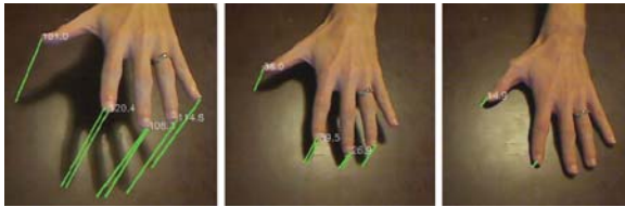
Figure 11: Tracking of the 3D position of multiple fingers (left). The displayed numbers give the height of each finger tip in millimeters. The green lines connect finger tips with the corresponding shadow points. If the hand moves closer to the interaction plane the detection of convex defects fails and the 3D position can not be computed (middle and right).
