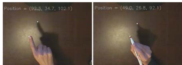
Figure 2: A selection/drawing operation using a single feature point defined as tip of the index finger (left) or tip of an external pointing device such as a pen (right).
