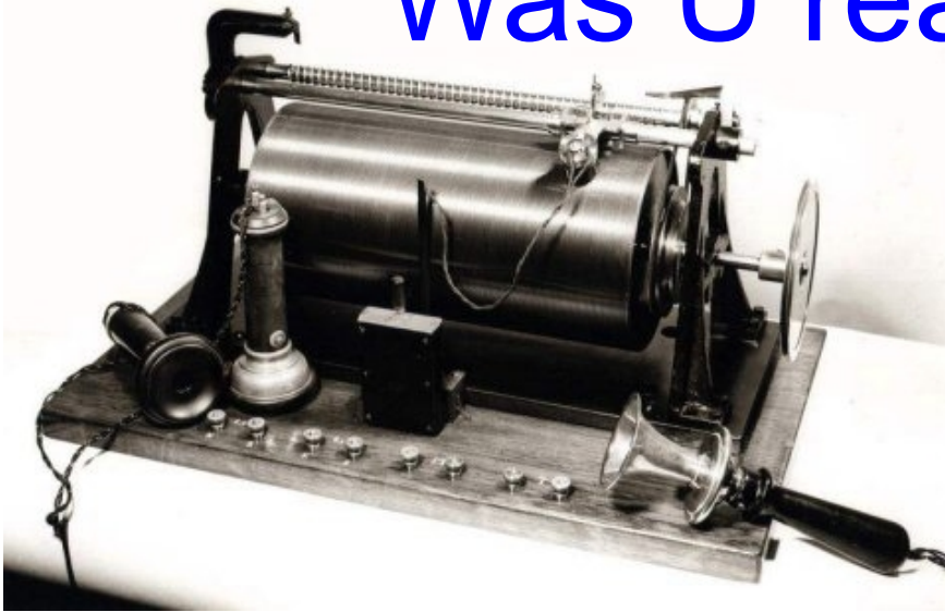
1898 Poulsen "Telegraphone" wire recorder (image from www.johansoldradios.se )
